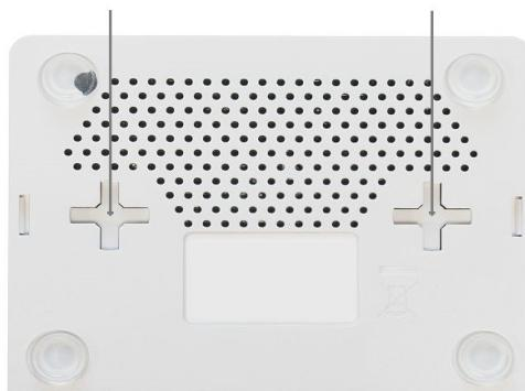
When mounting on the wall, please ensure that cable feed is pointing downwards. We recommend using Cat5/6 cable for our devices. The IP rating scale for this device is IPX0.
